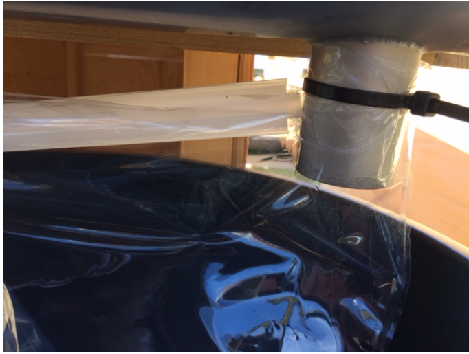
Figure S4 Sampling setup and attachment of PFA bags for sample collection to the stainless steel gutters. PFA bags were placed in plastic buckets for stability.
