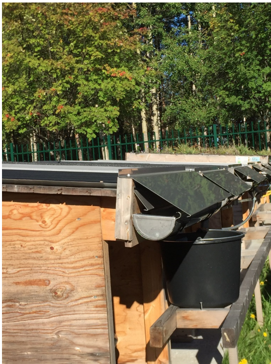
Figure S3 Sampling setup with stainless steel gutters for runoff collection and overlays for prevention of rainwater entry. Plastic buckets were used to stabilise the PFA bags used for sample collection.
