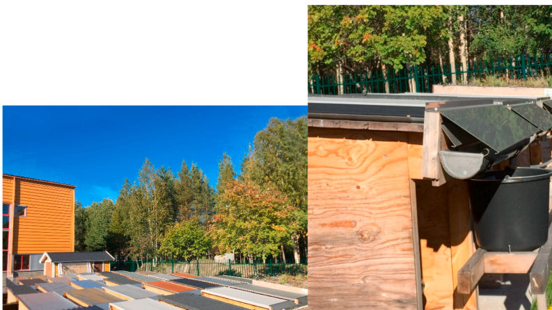
Fig. 2. a,b. (a) Overview of the test site of the open-air pilot study with different materials mounted on separate panels and (b) Experimental setup of the open-air pilot study, with stainless steel overlays and gutters collecting the runoff. The black buckets were holding the PFA bags.
