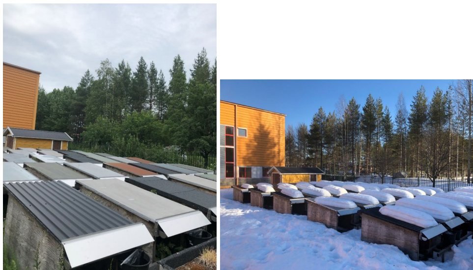
Figure 4 Pilot panels with PFA bags installed before a rain event (left) and during snowmelt runoff collection (right).
